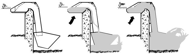
No flow until water level reaches elevation  $\mathbf{H}_{a}$ .
