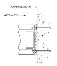
☐ Frame Mounted to Surface of Channel
