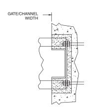
☐ Frame Embedded in Channel Wall
